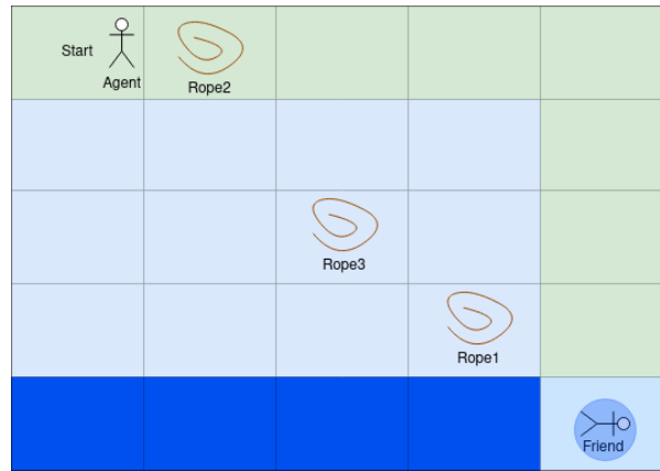
FIGURE 6.3. Frozen Lake environment Task 3: \varphi_3 = \diamond(R_1 \wedge \diamond(R_2 \wedge \diamond(R_3 \wedge \diamond F))) (i.e. eventually get the Ropes in order and then eventually get to Friend).
